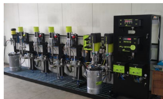
The installation of control boxes is in a non-explosive area.
